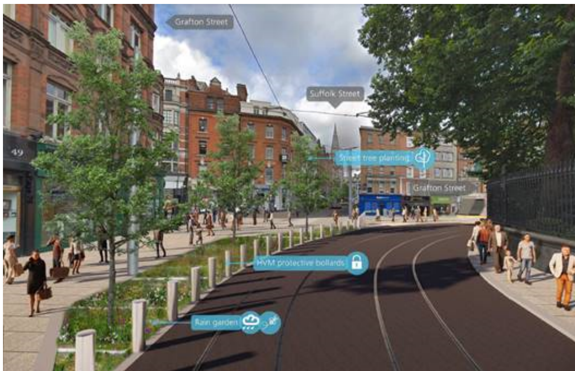
Figure 4 Example of previously proposed public realm designs for Dublin using SuDS. Source: DCC
